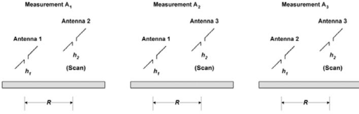
Fig. 3. Three site attenuation measurements using three different antennas in pairs
