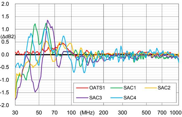
Fig. 9.  $\Delta dB2$  at each site using  $Hybrid_1$  and  $Hybrid_2$
