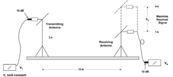
Fig. 2. Antenna arrangement of SSM
