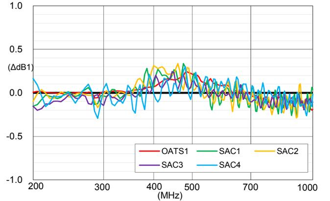
Fig. 6.  $\Delta\text{dB1}$  of LPD<sub>2</sub> measure at each site
