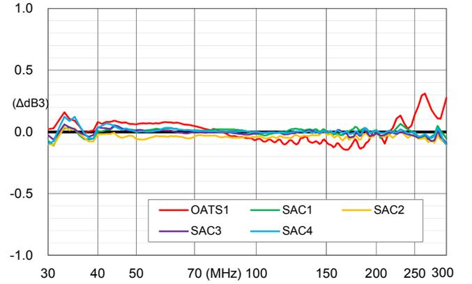
Fig. 10. Differences AFs ( $\Delta dB3$ ) for  $Bicon_2$  at each site and  $AF_{ref}$
