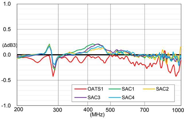
Fig. 11. Differences AFs ( $\Delta\text{dB}_3$ ) for LPD<sub>2</sub> at each site and  $\text{AF}_{\text{ref}}$
