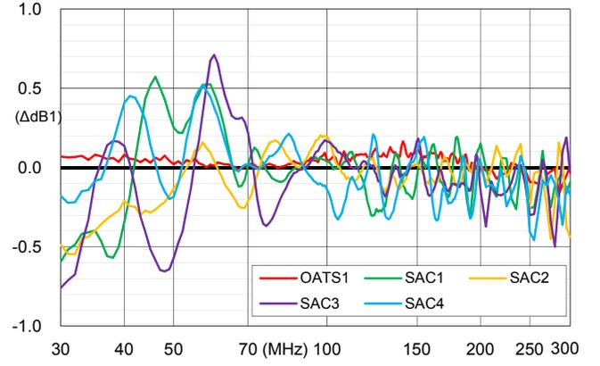
Fig. 4.  $\Delta\text{dB1}$  of Bicon<sub>2</sub> measured at each site
